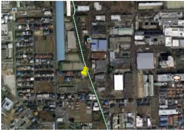
Figure 14. Result of positioning test with processing software in Google Earth. Accuracy is within 20 meters.
